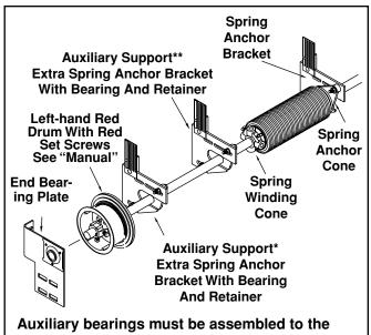
shaft before drums are put on shaft. \*Used on 20' [610 cm] or wider doors or doors 730 lbs. [331 kg] or greater. To be installed approximately 3" in from drum.
