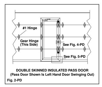
NOTE: Swinging portion of Pass Door on bottom section may need to be shimmed up during installation of upper sections to prevent gapping. (FIG. 5-PD)
